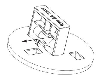
Fully open fuse holder and remove fuse. Replace with new fuse.
