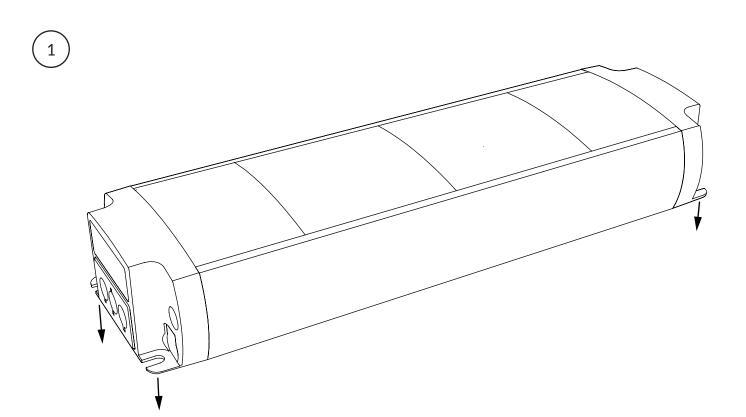
Attach unit to surface if needed via 4 alignment holes.
