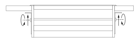
Place I-brackets against underside of desk, secure in position by tightening screws.
