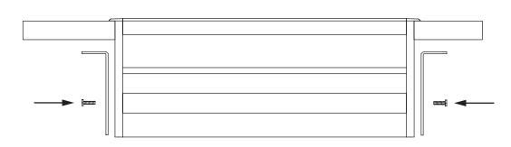
Loosely attach I-bracket to side of unit, fastening screws into nuts located in wall.
